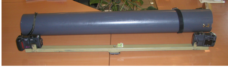
Figure 1. Two digital cameras, fixed on a metal bar (water level in the centre). Behind – the field carrying case
