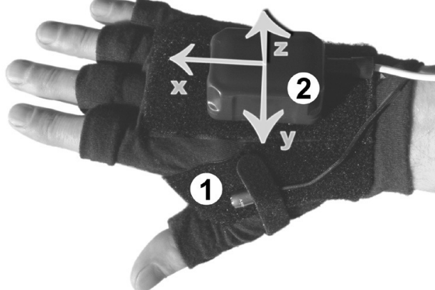
Figure 3.3. Glove used for data collection II with microphone (1) and accelerometer (2) together with axes definition.
