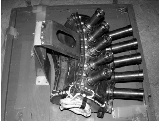
Figure 3.6 20° model of a real double annular combustor used in mid-power range stationary gas turbines [67]
