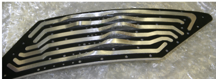
Figure 7.3: Cover with contoured negative element ensuring constant channel cross sectional area.
