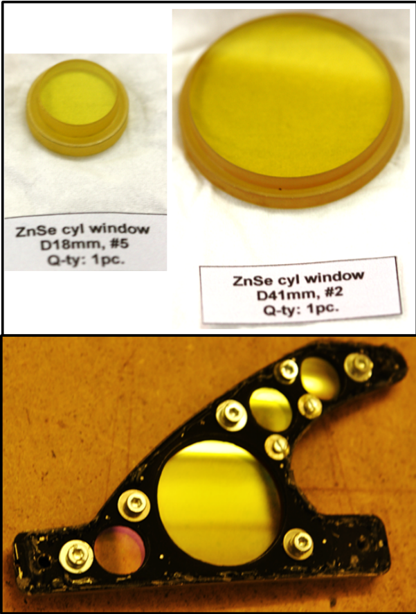
Figure 4.15: Top - pictures of the smallest D18mm windows (left) and largest piece of D42mm. The bottom part shows the assembly of the windows into the steel holder.
