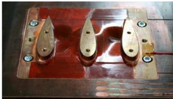
Figure 3.12: Contoured endwall case. Copper insert covered with the insulating Kapton layer.
