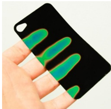
Figure 2.2: Example of a sheet of ThermoChromic Liquid Crystal reacting to the temperature of the hand holding it.
