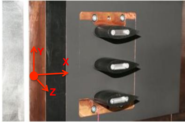
Figure 3.10: Test section (opened) of the facility. Three NACA profiles mounted on the isothermal plate.
