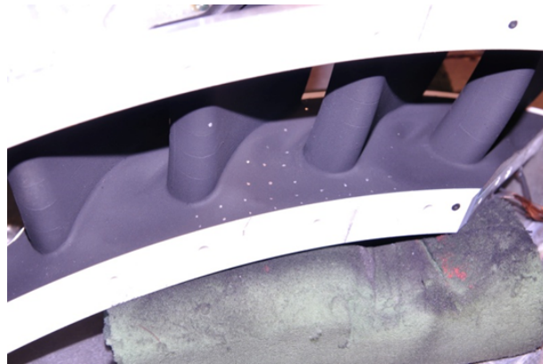
Figure 7.7: Heat transfer platform painted with high emissivity paint and with infrared markers on the endwall surface.
