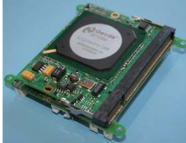
Fig.6.10. The x-board based, 40 g and 56x71 mm computer module
