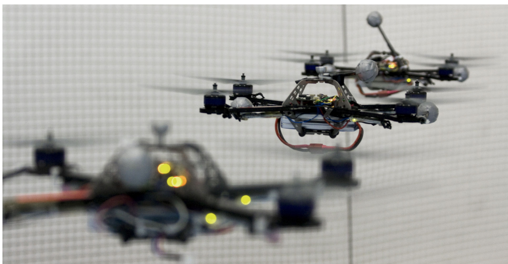
Figure 1.1 Quadcopters used for the experimental validation of algorithms. These vehicles measure approximately 35 cm from propeller center to propeller center, and weigh about 500 g.
