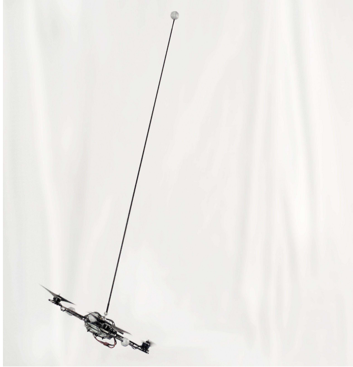
Figure 3. Photograph of experiments: The vehicle flying a circle while balancing the inverted pendulum.
