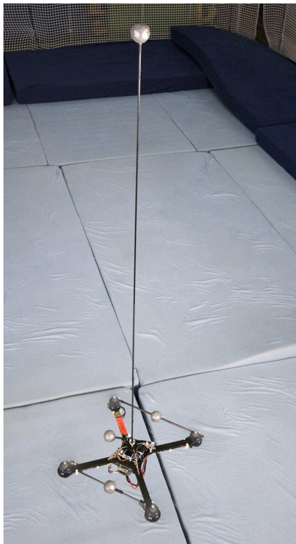
Figure 3. The quadrotor balancing the pendulum, at standstill. The mass center is about half-length of the pendulum.
