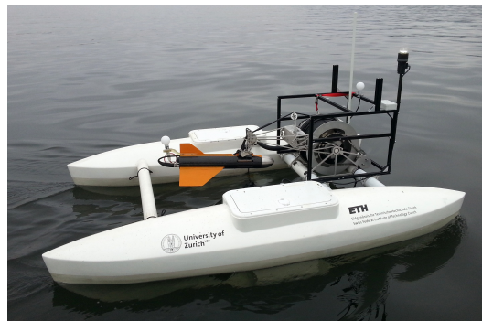
Fig. 1. The Autonomous Surface Vessel on Lake Zurich on a calm day. The YSI probe is mounted inside the black and yellow torpedo situated in between the hulls and is ready to be lowered into the water.
