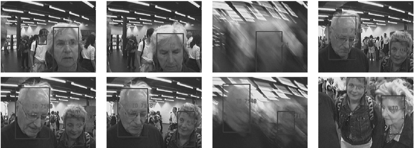
Fig. 4. Sequence of faces tracked by a RoboX at the Robotics exposition. From left to right and top to bottom, RoboX first tracks the face of a woman, then in the third image, it moves the eyes toward a man and tracks him until the next eye movement in the third image of the second row, where a third person appears.
