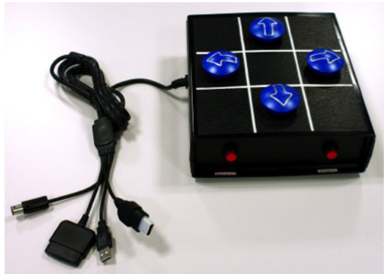
Figure 7. 1 Hand-held controller ( 20 x 20 x 60 cm)
