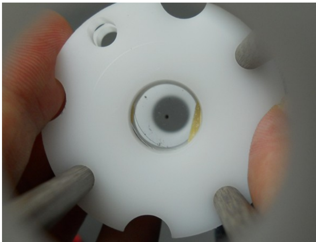
Figure E.1: A commercial Hg spectroscopy cell with 1 mm optical path length. The dark spot was observed after several hours to few days of exposure to UV resonance light. It turned out to be a opaque layer on the inner surface of the glass could be removed by heating the cell to 100 °C. The cell is shown on its mounting support. A droplet of metallic Hg is visible at the bottom of the cell.
