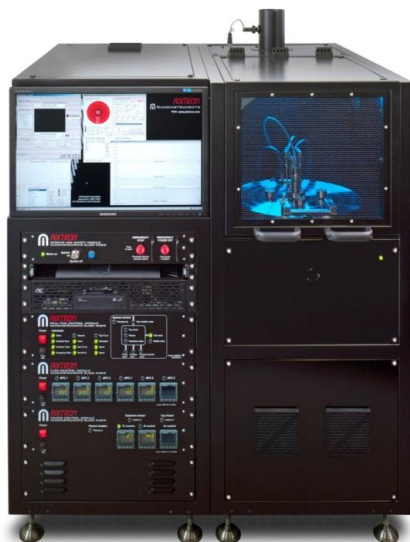
Figure 3.1. The cold-wall, vertical-flow CVD system by Aixtron, AG. All growths in this work have been performed by use of this system.
