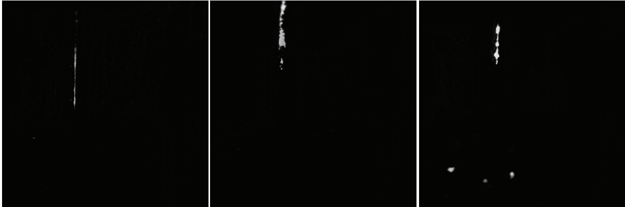
Figure 3.12: Ambiguous breakage events. The images are processed to remove unnecessary reflection around the aggregates for the purpose of appropriate detection. Breakups are ambiguous in the sense that fragments seem to be connected by thin parts rather than visibly separated from each other.
