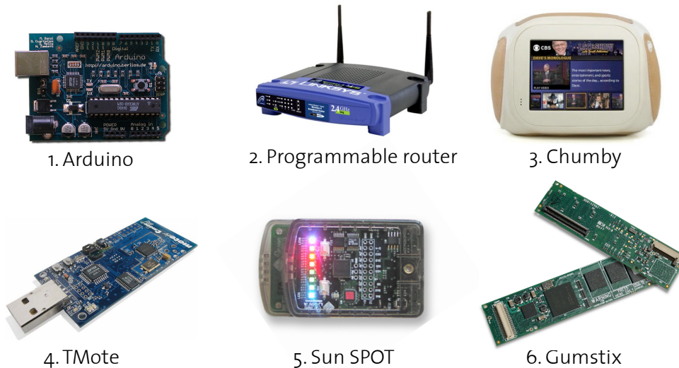
Figure 2.1: Various networked embedded devices (NEDs) that have been used in this thesis.
