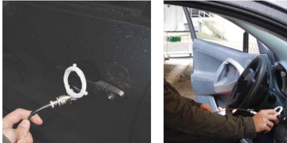
(a) Loop antenna placed next to the door handle. (b) Starting the engine using the relay.
