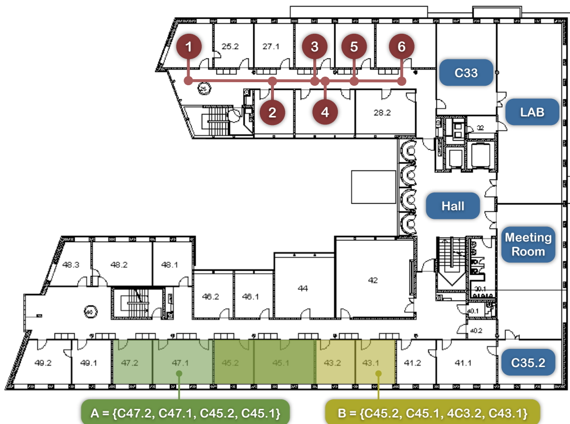
Figure 2.3: Different variations of symbolic location models (based on [10]).
