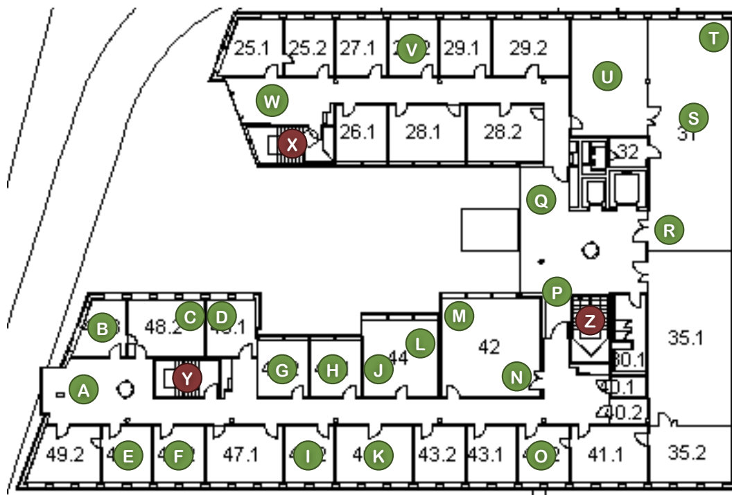
Figure 4.14: Points where measurements were taken. The labels A to W indicate on-floor measurements while X, Y, and Z indicate measurements that were taken on the stairs between the floors.
