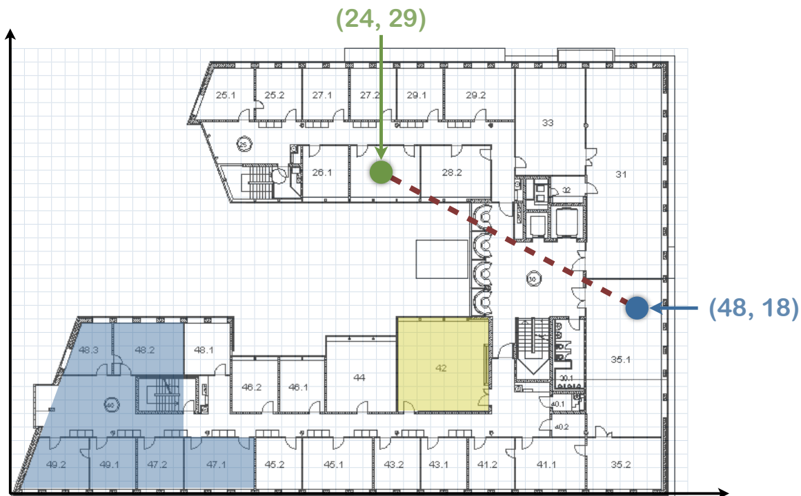
Figure 2.2: Example of a simple geometric location model using a local coordinate reference system.
