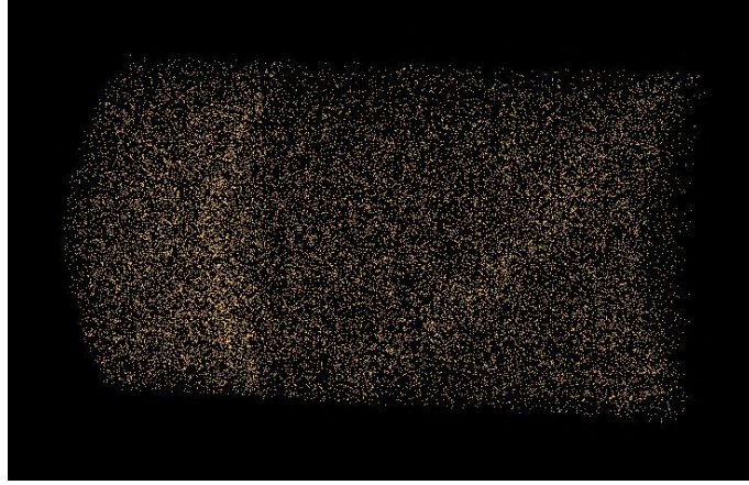
Figure 8: 3D point cloud of hydrogen atoms in evaporated sample tip, which has a length of \sim 120 nm and a diameter of \sim 60 nm.
