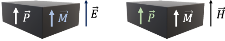
FIGURE 1.1: Visualization of the magnetoelectric effect, where an electric field induces a magnetization (M) and a magnetic field induces a polarization (P).
