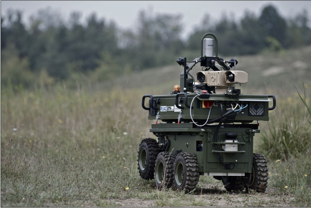
Figure 5.9: Photograph of Artor, a Search & Rescue robot specialized for outdoor applications.
