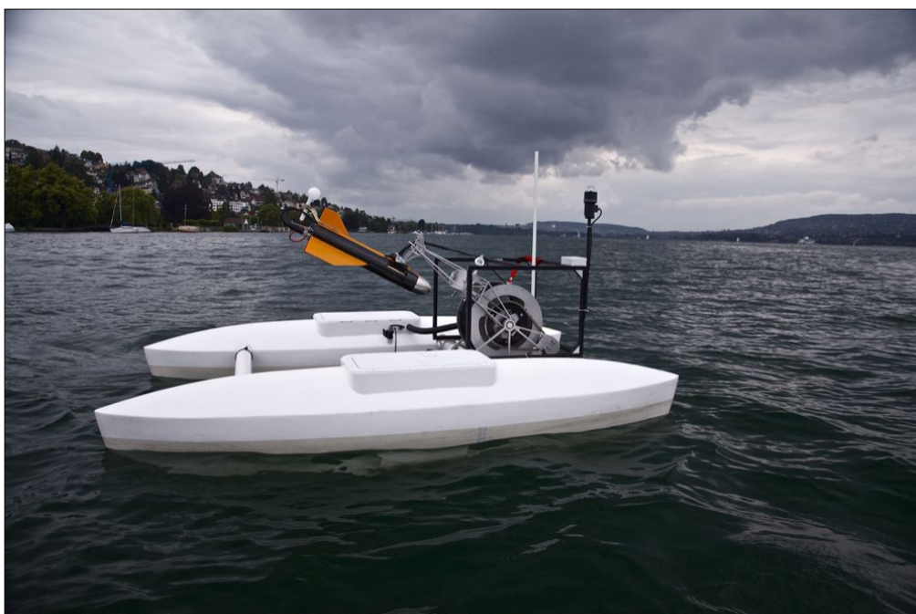
Figure 5.15: The autonomous surface vessel, named Lizhbeth, during one of its survey environment: pre-alpine Lake Zurich, Switzerland.
