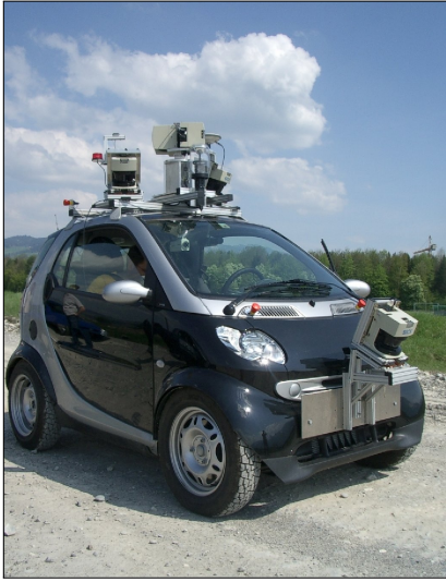
Figure 5.17: The autonomous car, named SmartTer, with its suite of five Sick LMS-291 laser rangefinders. Larger wheels were installed to allow off-road driving.
