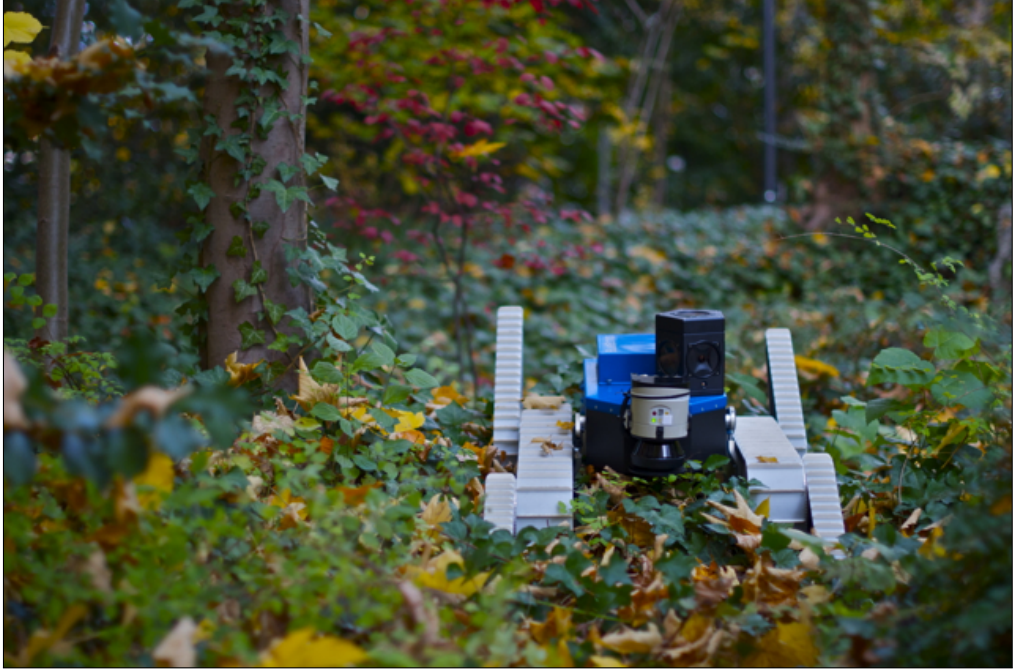
Figure 5.1: Photograph of NiftiBot, the main platform used for Search & Rescue demonstrations.
