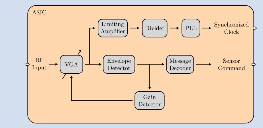
• Integrated in a bulk **65nm CMOS** technology in an area of **1.5 mm<sup>2</sup>**
