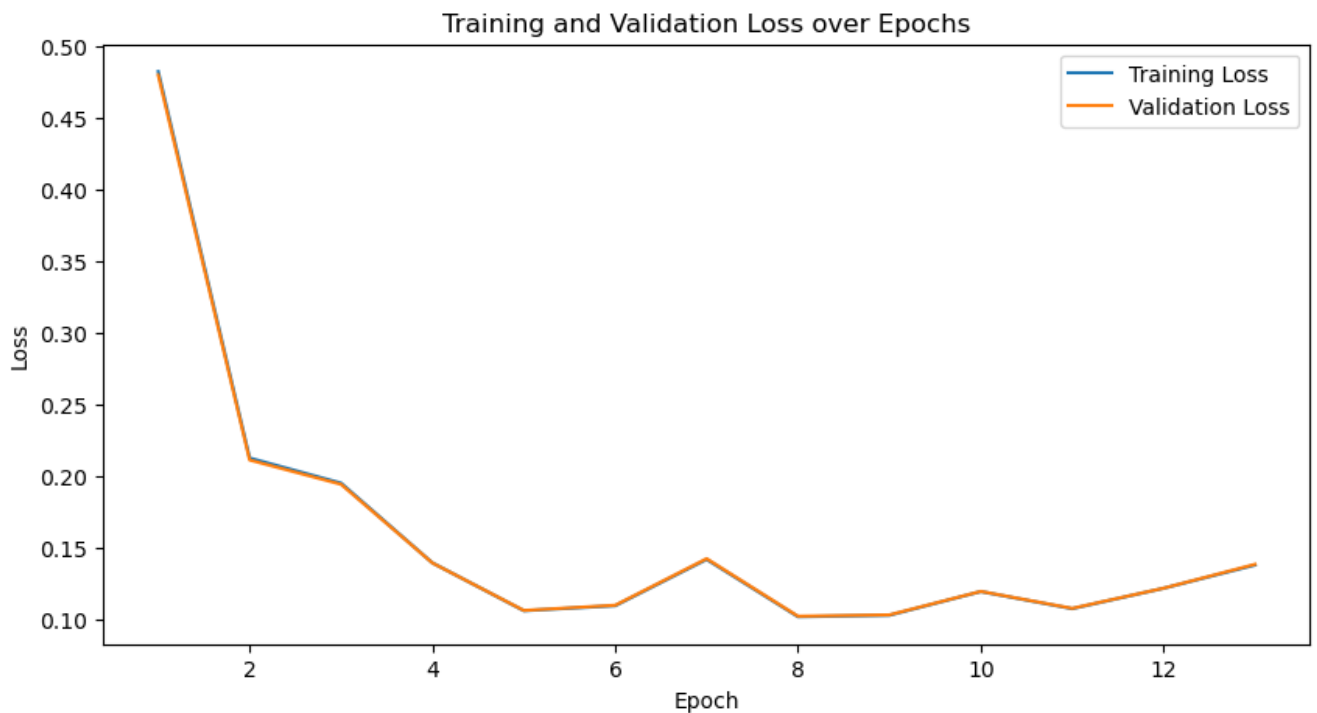
Figure 4.1: Training and Evaluation error for the FFNN Simulator
