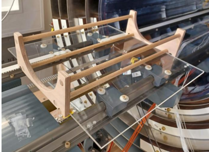
Figure 7.3: The wooden UCN guide mount, placed on top of the gradiometer trolley.
