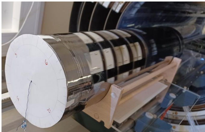
Figure 7.4: A UCN guide on the gradiometer trolley. A clock face is attached to the marked side (which enters the gradiometer last), defining the angular positions. The position shown in this figure is position 8. Since the paper clock face produces a magnetic signal, it was removed before the measurement.
