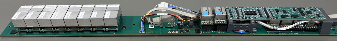
Figure 2.14: Full assembly of the SDIP3, including eight detector head modules on the left, the attached SBTV3 PCB, SSPD PCB and DC-DC power converters on the right, as well as the Kintex-7 FPGA towards the center. Not visible is the 10G SFP+ Ethernet connector and glass fiber, hidden below power converters and the SBTV3 PCB.
