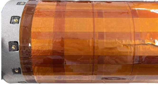
Figure 2.20: Copper-Kapton shield surrounding the inner cylinder of SAFIR-II. Each copper strip is cut to be no larger than 2 cm in width. While all strips overlap such that no gaps in the cylindrical structure are present, the strips are electrically insulated from each other by the layers of Kapton.
