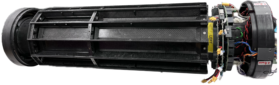
Figure 2.18: Carbon fiber mechanical support structure of the SAFIR-II insert. The 12 ‘caskets’ in the central part are additionally covered with carbon fiber lids (not visible here), with the entire structure being surrounded by carbon fiber covers as well. Already mounted and visible on the right are the SPPD, SBD and SFCD ring boards.
