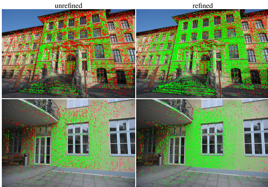
Figure 2.6.: Triangulation with dense correspondences. We show reprojections of 3D points triangulated with dense matching for two scenes (top and bottom) reconstructed with (right) and without (left) refinement. The points are colored as accurate (in green ●) or inaccurate (in red ●) wrt. the ground truth for a 1cm error threshold. The refinement yields many more accurate points and can handle extremely dense reconstructions.
