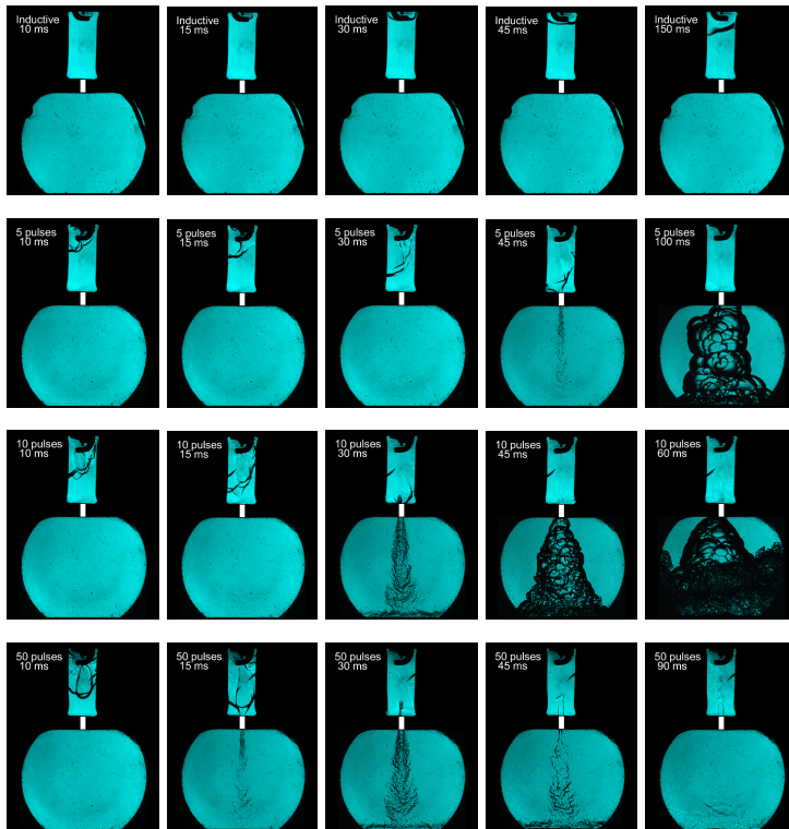
Figure 6.12: Ignition sequence in the PC and in the MC using the inductive and NRPD ignition system with 5, 10, and 50 pulses. 10 kHz, 12,4 bar, 90 °C, \lambda = 1.8 . Laminar conditions in the PC.
