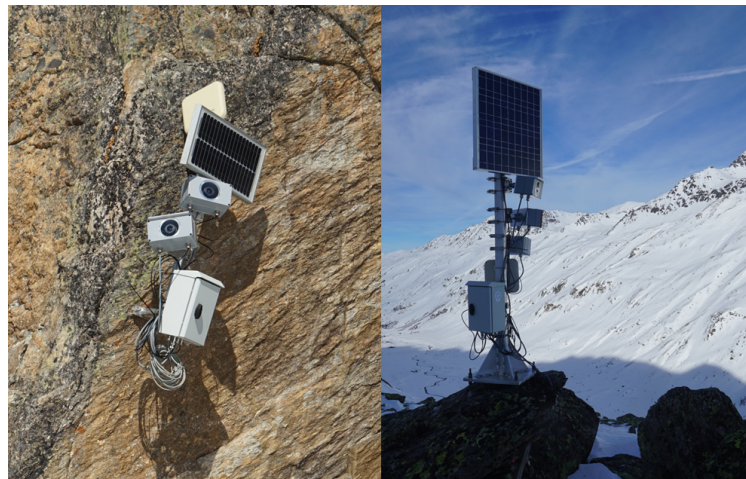
Figure 20.2: The stations in the Dischma Valley were either bolted to rock faces (left; Lukschalp) or mounted on a mast (right; Sattel). They host two to three cameras and all infrastructure necessary to ensure power supply as well as data acquisition and transmission.
