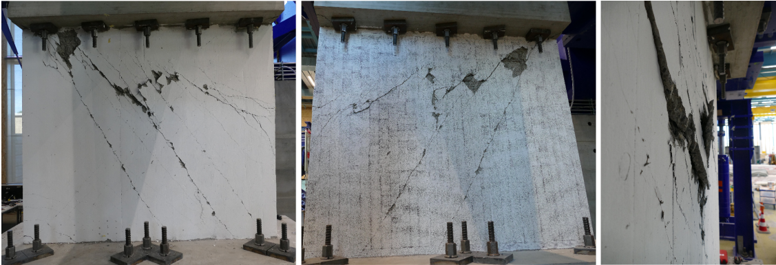
Figure 5.23: Final state of specimen HSW02 at the end of the hybrid simulation with 2.75 scale factor
