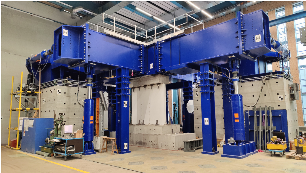
Figure 3.7: ETH MAST Facility with specimen SW04 installed in it.
