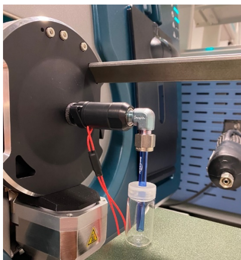
Figure 61: Exemplary setup for the use of DBDI-MS. An EO is placed in a headspace vial, incubated and directly coupled to the source via a GC liner. Image taken from Raeber et al. 21
