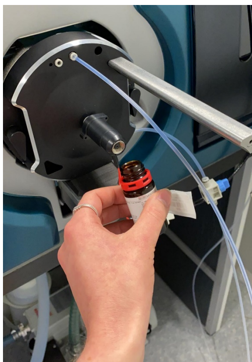
Figure 6: Direct sampling of an EO using a LTP-source. Operating at atmospheric pressure, the open architecture allows direct sampling. Photo was taken by the author.
