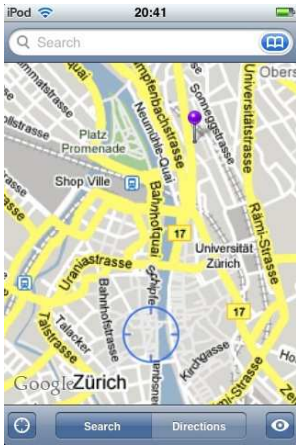
Figure 4: Location spoofing attack. Location displayed by the iPod in city downtown (marked by a circle) at about 1 km distance from the iPod’s actual position (marked by a pin) at university campus (caused by an AP impersonation/replacement attack).
