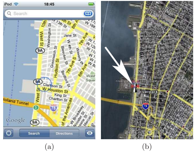
Figure 3: Location spoofing attack. (a) Location in New York City (circle in the center) displayed by an iPod physically located in Europe (caused by an AP impersonation/replacement attack) (b) Physical location of impersonated APs (indicated by the arrow and displayed using Google Earth [3]).
