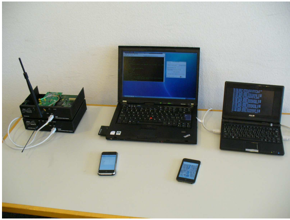
Figure 2: Equipment used in our experiment. The iPod and iPhone are the LNs, the laptops are used to impersonate access points (APs), and the software radios are used to jam legitimate APs.
