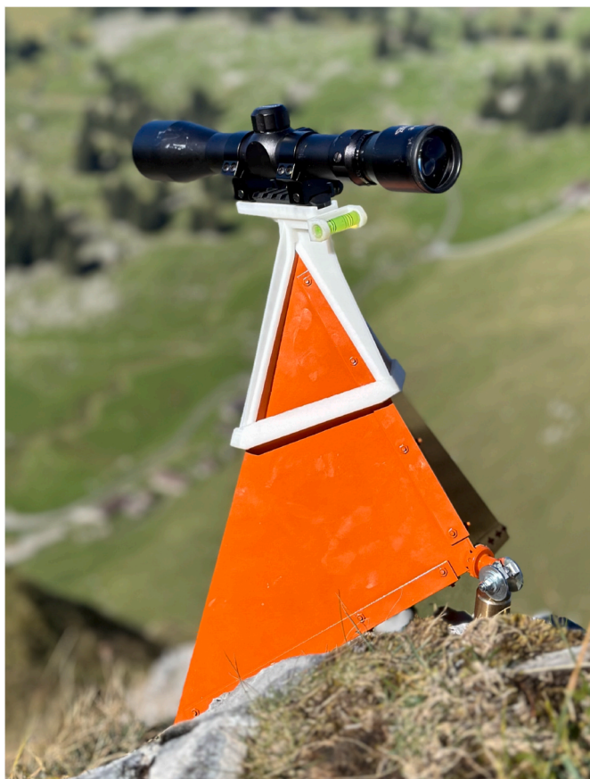
Fig. 2. Installed mmCR with the 3d-printed mounting system for attaching the telescopic sight.
