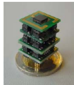
Figure 1. The Sensor Cube hardware platform developed by IMEC: Layers from top: Radio, Microcontroller, Power and Sensor Module. A 2€coin provides a size reference.
