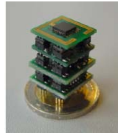
Figure 1. The Sensor Cube hardware platform developed by IMEC: Layers from top: Radio, Microcontroller, Power and Sensor Module. A 2€coin provides a size reference.
