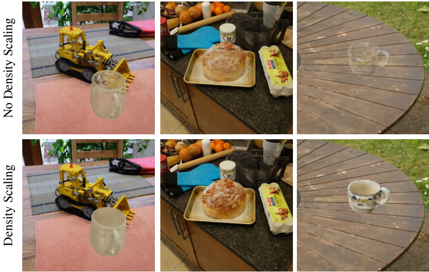
FIGURE 5.7: The effect of density scaling on fusing object and scene. When the object NeRF scale is not accounted for in the volumetric rendering, the object is not properly displayed in the rendered views.
