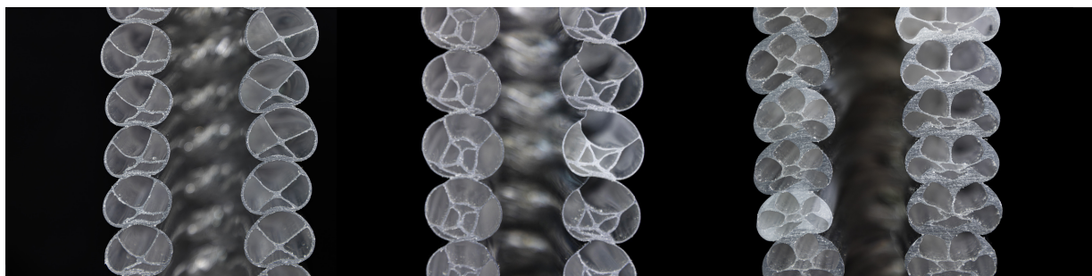
Figure 5.10: Section of 3D printed samples. A) Quad. B) Crosshair. C) Tube in tube.
