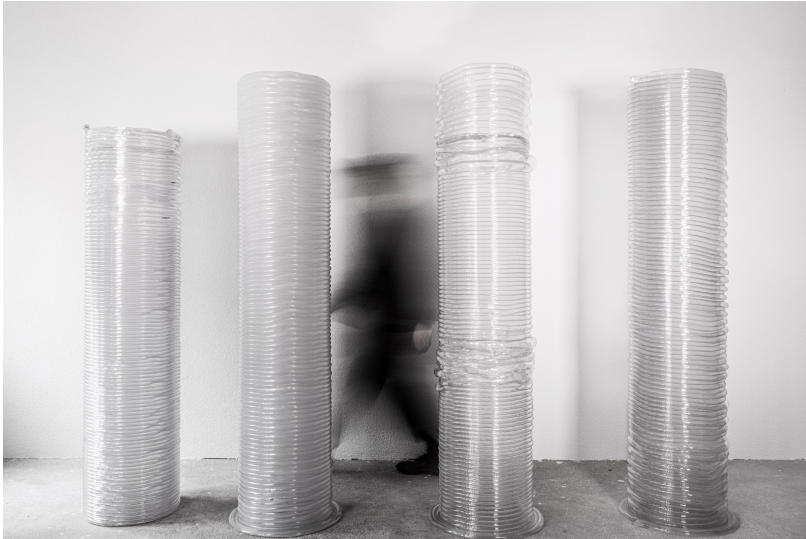
Figure 4.14: Series of 40cm diameter cylinders printed at different layer heights. The final demonstrator (right) is 2 meters tall, and the print time is 1:54 hours, weight 10.3kg.
