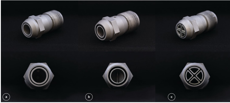
Figure 4.4: Different nozzles types, prototyped using 3DP of aluminum.
