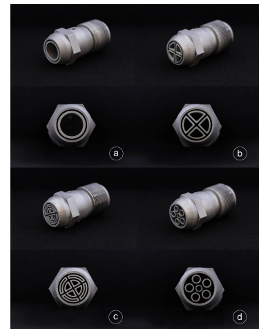
Figure 5.4: Different nozzle types, prototyped using 3DP of aluminum.
