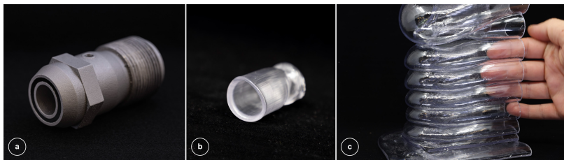
Figure 4.12: HC3DP nozzle with a 24mm orifice and a 2mm wall thickness. (b): Extruded PETG bead. (c): 3D printed sample, cut, with a hand to represent scale and transparency.
