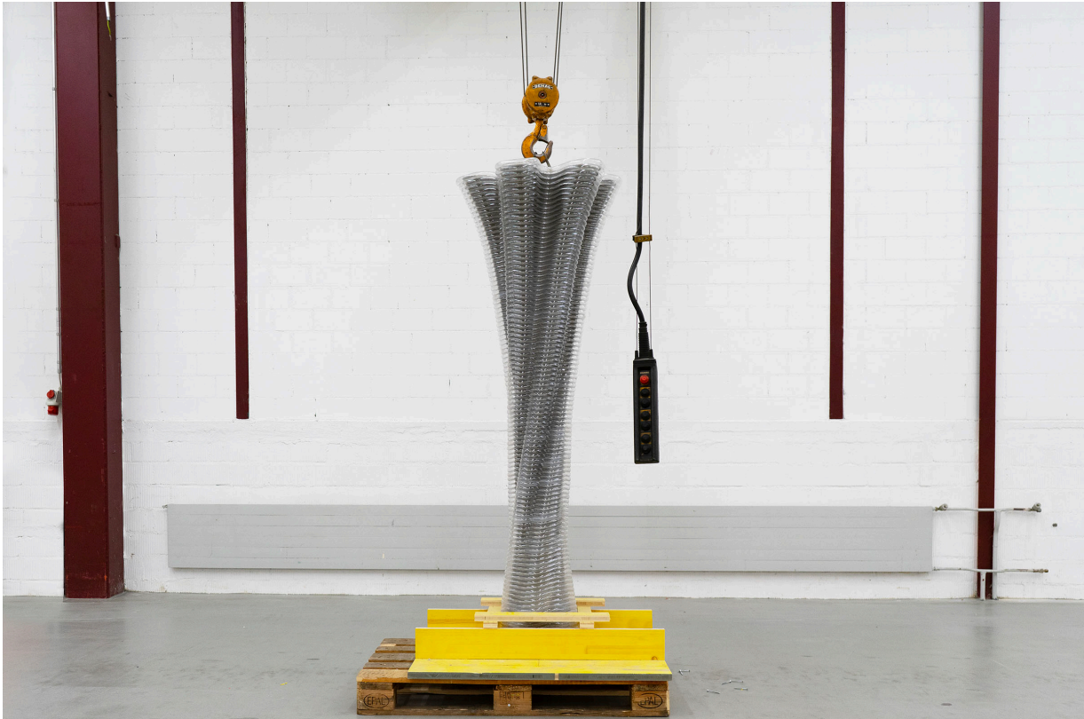
Figure C.1: 2.1 m tall concrete column cast into HC3DP formwork.
