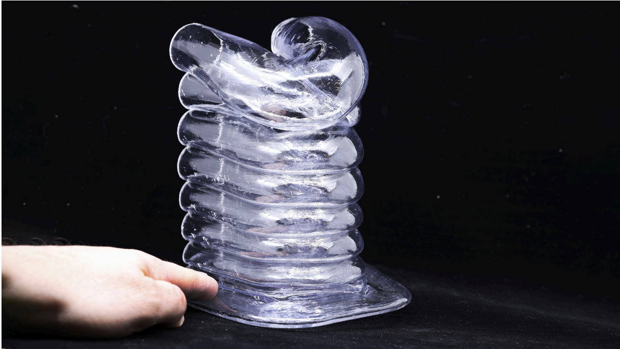
Figure 5.1: Large-scale HC3DP samples. Layer height 18mm, layer width 24mm.
