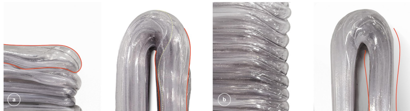
Figure 4.16: (a): overinflation due to constant internal air pressure. (b) successful print due to active control of air pressure. Red indication overinflated bead. Yellow indicates the twisting of the bead due to constant tool orientation.
