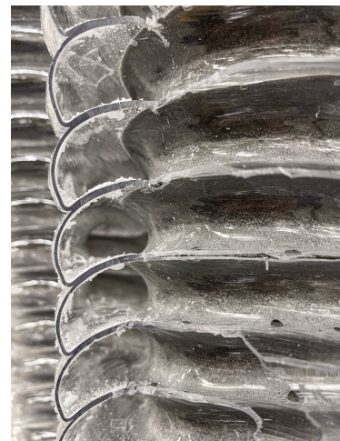
Figure C.2: Close-up during demolding of HC3DP formwork.
