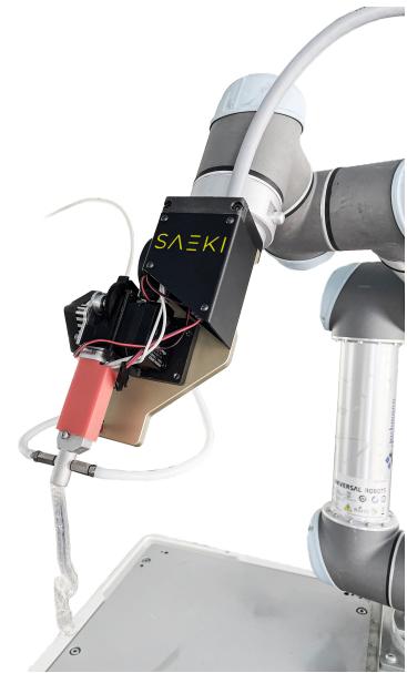
Figure B.1: UR-5 co-bot with a filament-based HC3DP system attached.
