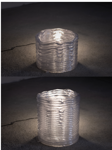
Figure 5.16: Non-planar HC3DP, the print failed after a height of 250mm. B) Non-planar HC3DP, printed to the end, as the undulations in Z directions are less strong.
