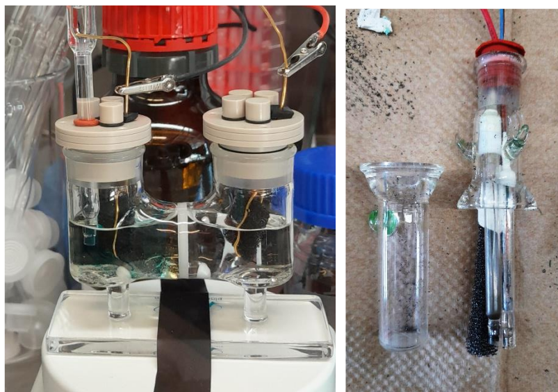
Figure 3. Pictures of preparative electrolysis setups in a divided (left) and undivided (right) cell with RVC electrodes.
