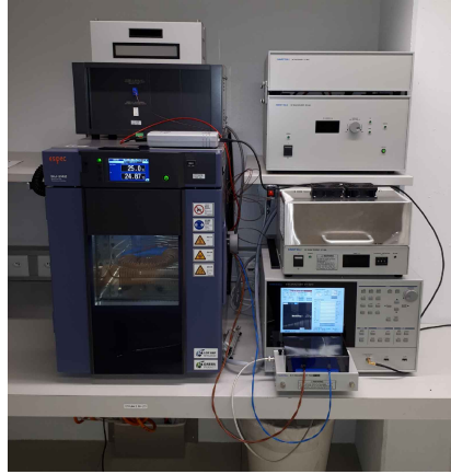
Figure 3.25: Core loss measurement setup.
