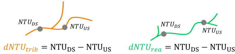
Figure 2.6: Differences in turbidity ( dNTU ) calculated as the upstream turbidity subtracted from the downstream turbidity. The locations of upstream and downstream turbidity are shown in the two panels: LEFT for tributaries and RIGHT for river reaches between two tributaries.
