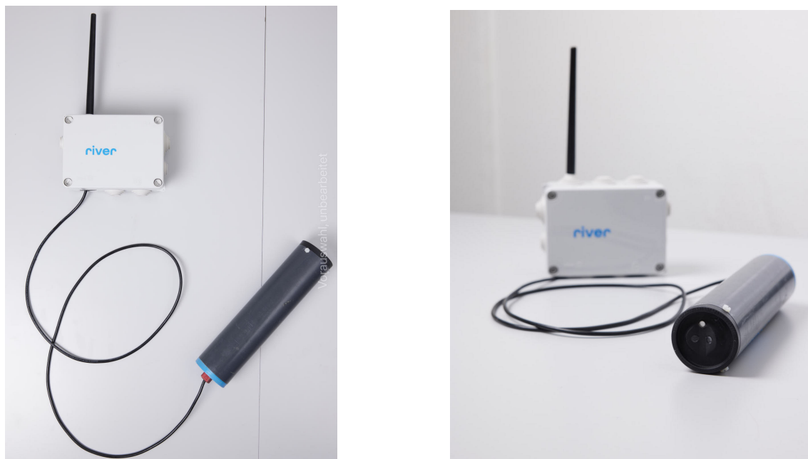
Figure 6.1: The latest version of our SSC sensor, the HydroHeidi. The box contains the battery and the LoRa module and the electronic components are inside the PVC tube.
