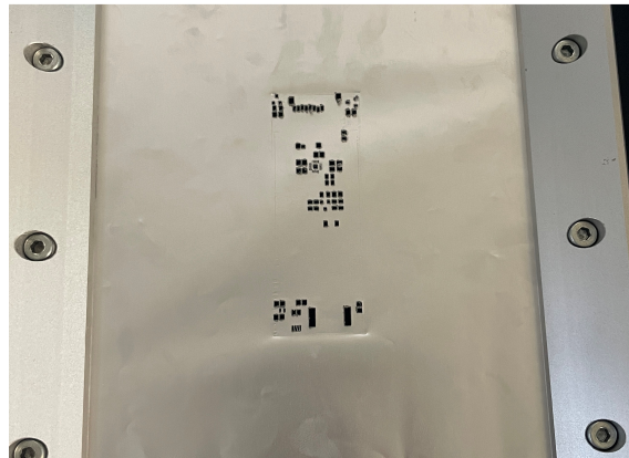
Figure 4.2: Makeshift stencil for solder-paste made with a laser cutter
