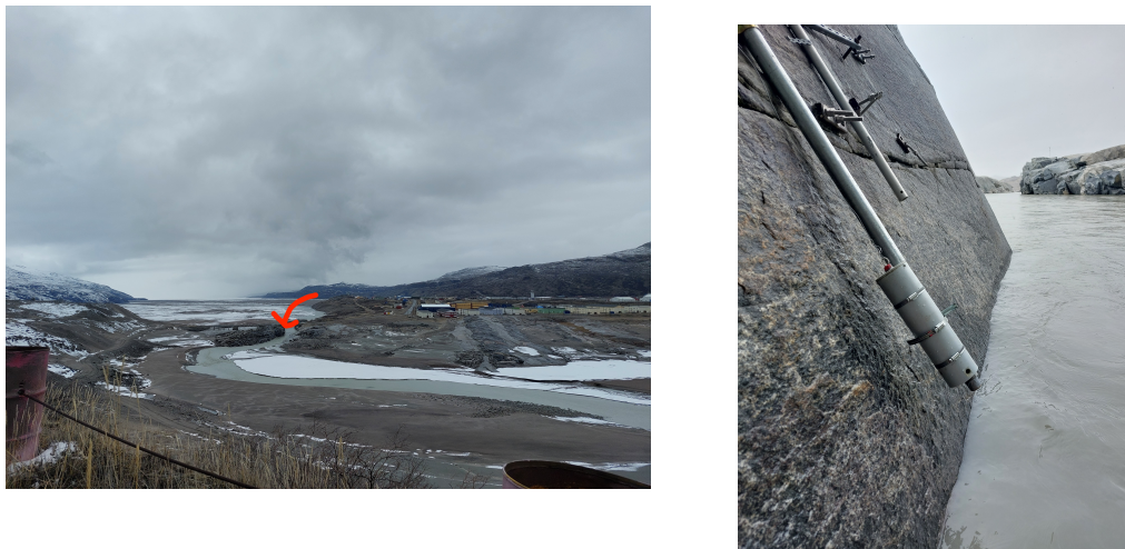
Figure 6.2: LEFT: The GlacierGuard installed on a proglacial stream in Greenland. The red arrow shows the installation location. RIGHT: A closer look at the GlacierGuard sensor installed on a bridge along a Greenland proglacial stream (Image by Ian Delaney).
