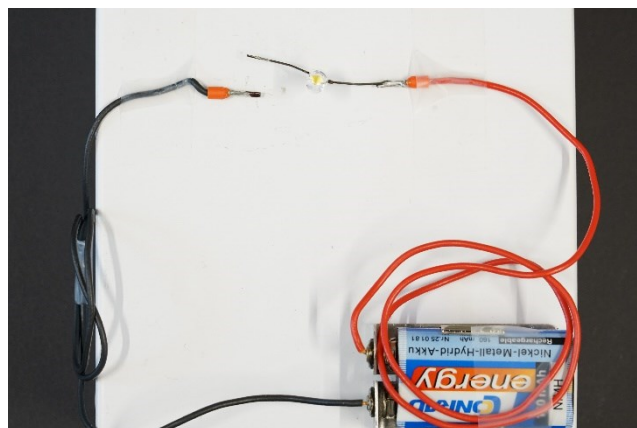
Figure S21. Electric circuit composed of a battery and LED.
