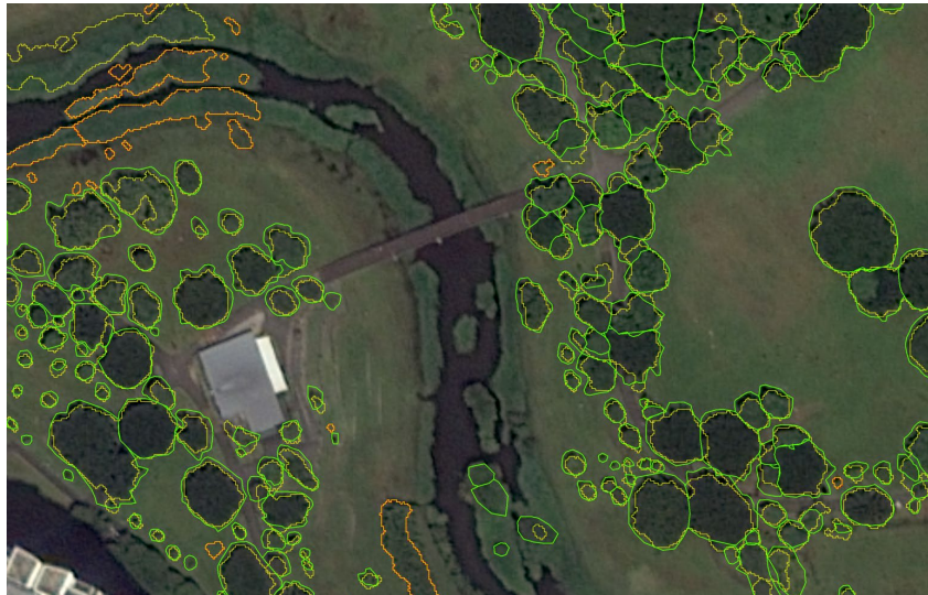
Figure 8. Satellite image at 0.5 m resolution. Manually delineated tree crowns are indicated in green, predicted crowns in yellow, and false positives in orange. Omitted: green instances with no corresponding prediction.
