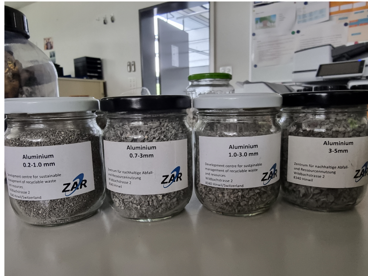
Figure 2.7. Sorted aluminum recovered from bottom ash. Zürich, Switzerland 24.05.2024
