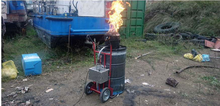
Figure 2.3. Commercial engineered barrel incinerator. Sourced from: Mavi Deniz .
