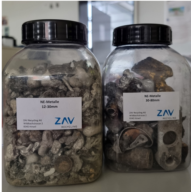
Figure 2.6. Large metal chunks recovered from bottom ash. Zürich, Switzerland 24.05.2024
