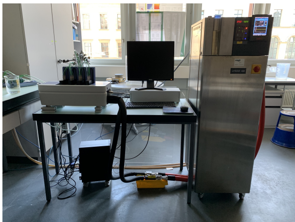
Figure 2.10 Ice nucleation setup, comprising Crystal16 instrument (left), desktop computer (center) and thermostat (right).
