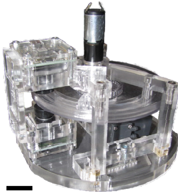
Figure 2.1. Latest version of the CellSorter for medium to large biological entities. Black bar indicates 20 mm.
