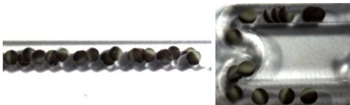
Figure 2.2. Results of oocyte rotation experiments. Each 3 rd frame of the experiment's movie was superposed to observe movement. (left) Channel with structured ground. (right) Vertical fall with induced rotation.
