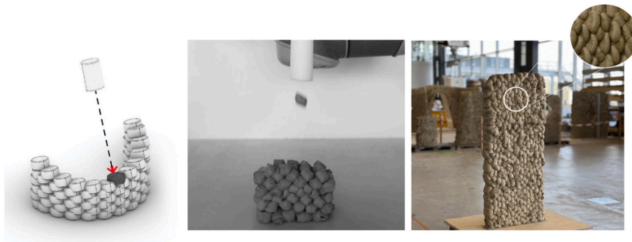
Fig. 4. (left) Visual representation of the high-speed discrete deposition method (adapted from [58]). The process convert kinetic energy into plastic deformation, enhancing adhesion between individual blocks (middle) [58]. The process was upscaled from the prototypical scale, enabling the production of large-scale prototypes fabricated at ETH, Zürich [61–63].
