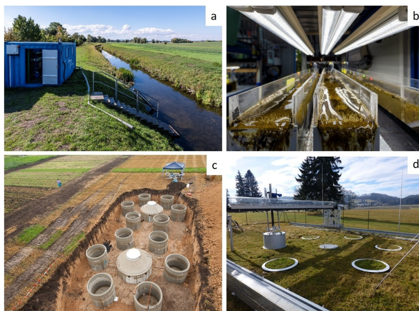
Figure 2. Examples of some of the TERENO experimental infrastructures: (a) MOBICOS container at an agricultural river side, (b) linear flumes within a MOBICOS container, (c) construction of a SoilCan lysimeter site, and (d) robotic system to measure soil greenhouse gas exchange on SoilCan lysimeters. Image sources: (a)–(c) André Kuenzelmann and UFZ, (d) TERENO.
