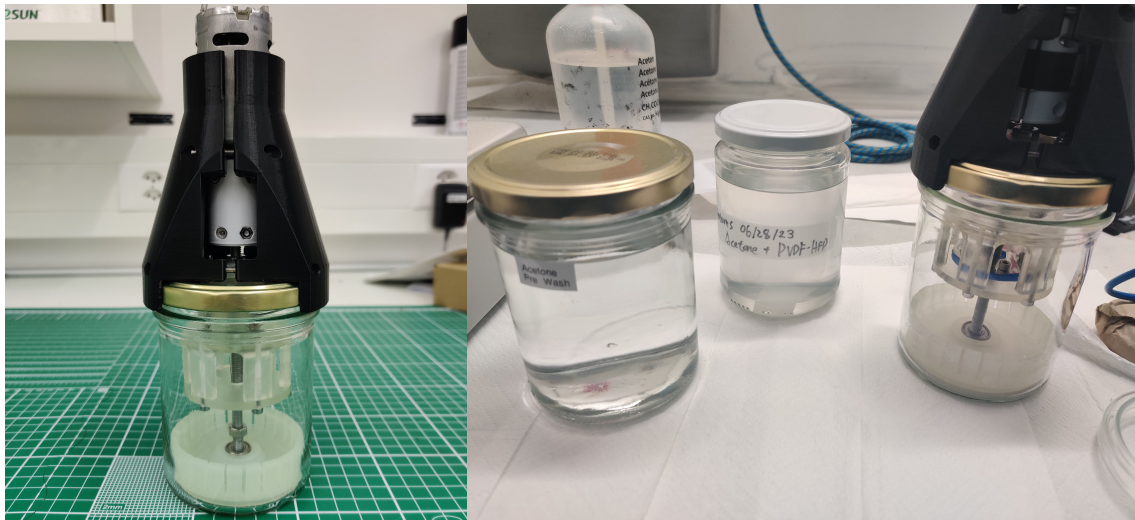
Figure 14: The spinning machine and the dip-spin-coating setup. The samples are installed into the spinning cage, dipped in the PVDF-HFP solution, and spun in the jar.
