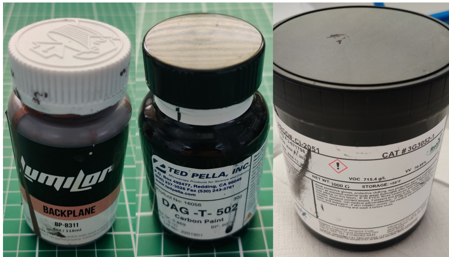
Figure 8: Three available conductive paints. From left to right: copper-based Lumilor backplane BP-B311, carbon-based carbon paint DAG-T-502, and carbon-based paint CI-2051.
