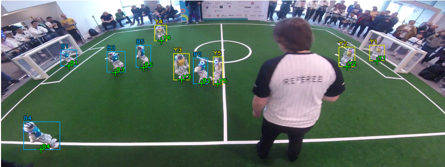
FIGURE 5.2: Visualization of robots identified by the tracker. The tracking result is represented by bounding boxes and IDs at their top. Ground truth positions are represented by green crosses and corresponding green IDs.
