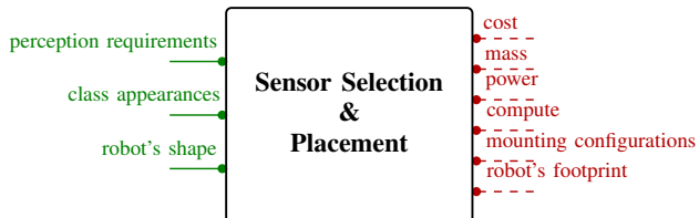
Fig. 15. The Sensor Selection and Placement MDPI which is the composition of the Coverage, Mounted Perception Pipelines and Perception Pipelines MDPIs.
