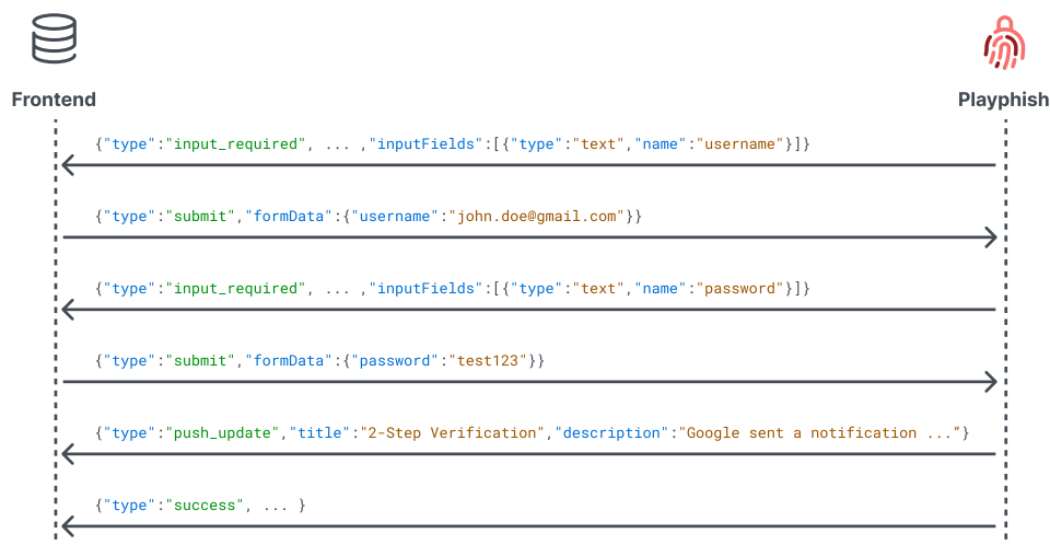
Figure 5.5: Messages sent through the WebSocket protocol between the frontend and Playphish. The corresponding screenshots are shown in Fig. 5.4.
