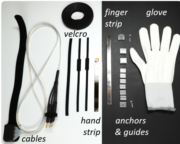
FIGURE 4.4: Assembly of the ES brake, 3D printed guides and attachments fastened to thin nylon glove using velcro.
