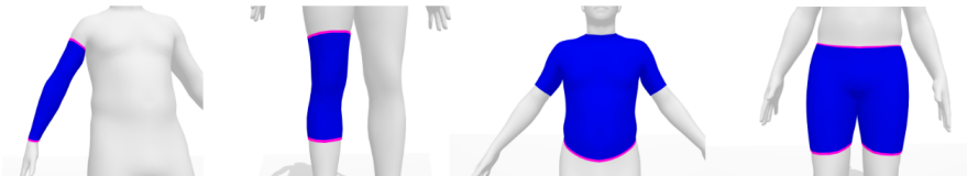
FIGURE 5.6: A range of garments designed with our tool. Pink areas represent attached areas. All garments start in a fully reinforced setting, which is represented with opaque blue color.
