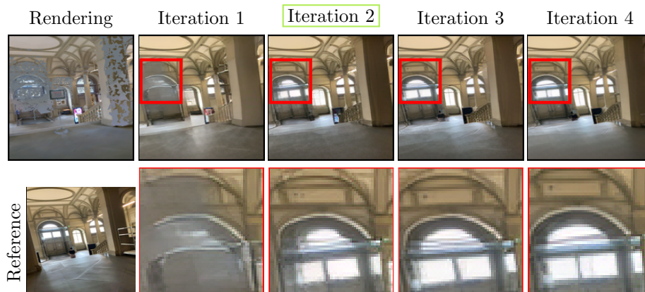
Figure 7.7: Visual improvement with iterative refinement. Refining the result over several iterations helps the correspondence matching in presence of large artifacts.
