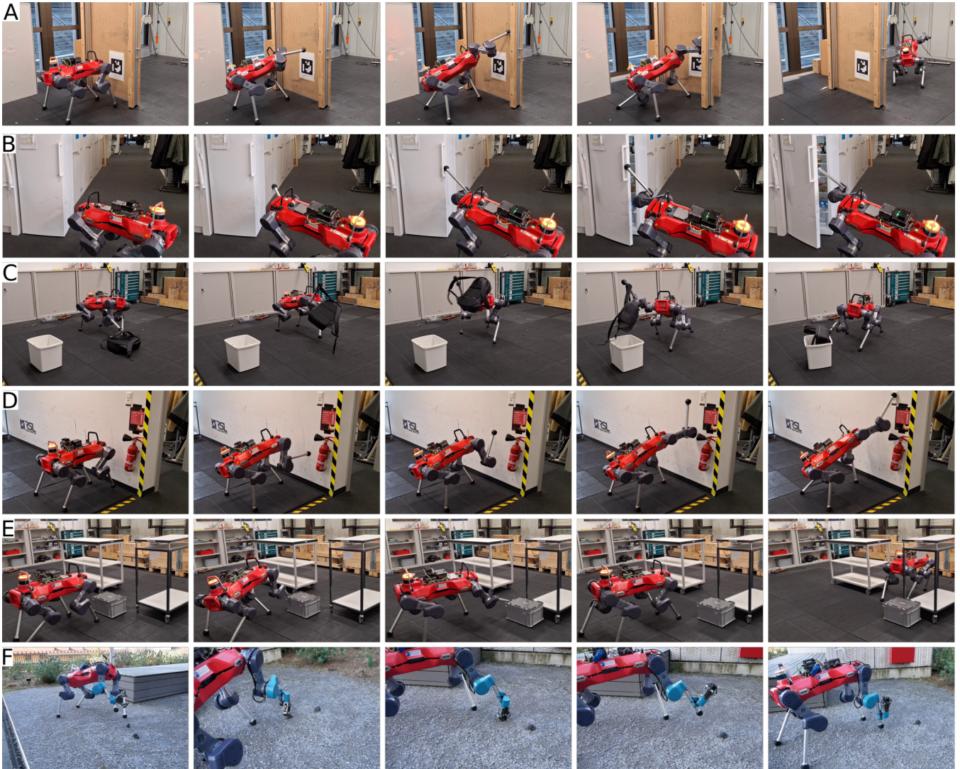
Fig. 4: Our controller enables numerous real-world manipulation tasks: (A) The robot opens a push door. (B) The robot opens a fridge. (C) The robot lifts a backpack and transports it to a box using a tripod-hopping gait. (D) The large workspace of the controller allows pressing a button far above the robot’s base. (E) The controller can be used to push obstacles out of the way. (F) With an additional gripper, the robot can collect rock samples.
